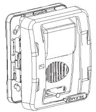
To remove bezel, grip both sides of bezel and pull in a download and outward motion.
