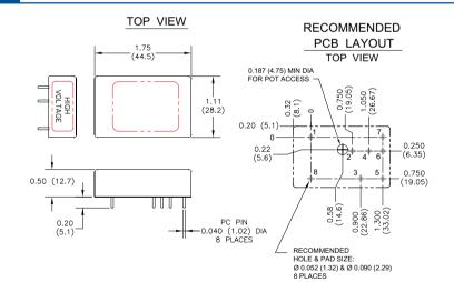
Description 5Vin 12Vin Pin Function VOUT High Voltage Output Ground to Pin 8 1 2 VPGM Voltage Programming Input, <150uA 0 to +2.048V 0 to +5V 3 SGND Signal Ground [For VPGM, VIN, VMON] Low Voltage Ground Voltage Reference Output, +/- 1% , 1 mA 4 VREF +2.048V +5V 5 CGND Case Ground Case Ground 6 VIN Input Voltage +4.75 to +5.25V +11.5V to +15.5V 7 VMON Voltage Monitor Output, 1mA, scales to 0 to 100% Vout 0 to +2.048V 0 to +5V 8 HV RTN HV Output Return Ground for Pin 1
