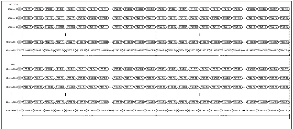
Figure 75 : Pixel Remapping for Color Binning
