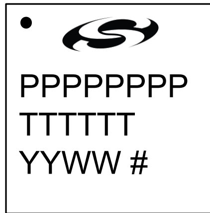
Figure 6.3. QFN28 Package Marking
