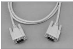
DB9 Data Switch Cable Wired Pin to Pin
