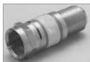
'F' Voltage Blocking Coupler Blocks DC and Low Frequency AC Power-Bandwidth: DC to 1 GHz, Return Loss 25db, (M) to (F)
