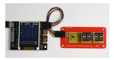
Starting the GUI and connecting to the  $I^2CD$ river on COM16 shows the temperature sensor at address 48 and the two display modules at addresses 14 and 15.
