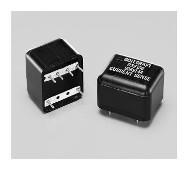
This Coilcraft current sense transformer is intended for use in measuring 50/60 Hz line currents from 0.5 to 20 Amperes rms. Typical application shown below yields an output of 0.1 Volt per Ampere. The output voltage may be changed by adjusting the value of the terminating resistance ( $R_T$ ). These parts also can be used to measure 400 Hz line currents.
