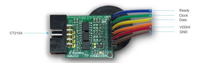
Figure 1.1: CT001 Isolation Streaming Board Connection
