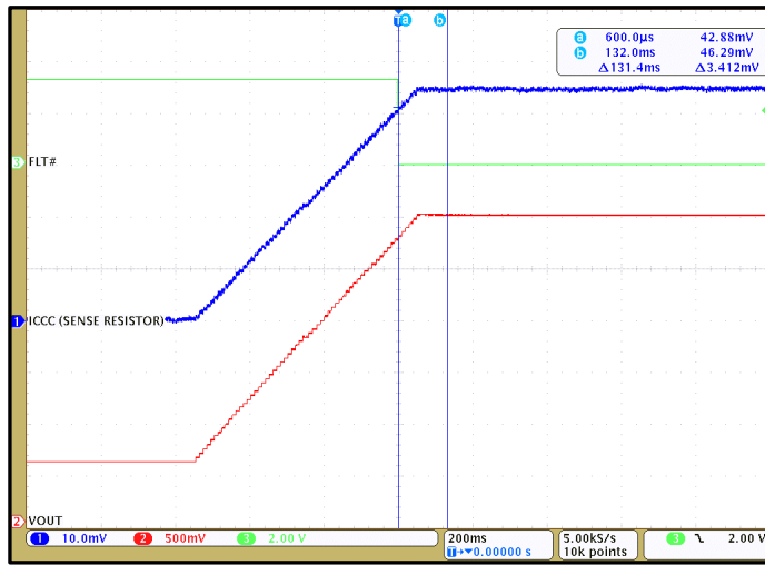
Figure 11. CT431 OCD enabled at 110% of +50 A DC and FLT# is LOW
