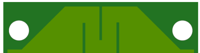
Figure 19. PCB Trace Design to Generate Differential Magnetic Field for CT452 to Measure
