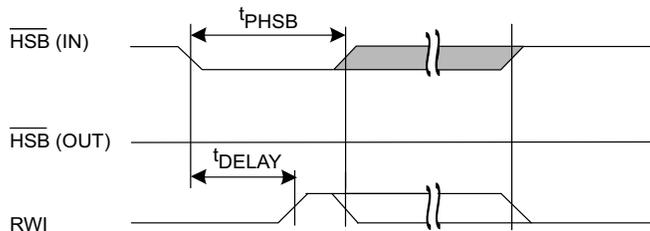
$\overline{HSB}$  pin is driven HIGH to  $V_{CC}$  only by internal 100 K $\Omega$  resistor,  $\overline{HSB}$  driver is disabled
