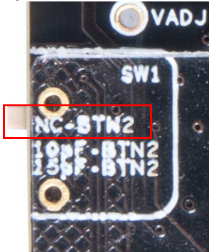
Figure 3-19. SW1 Slide Switch in NC-BTN2 Position
