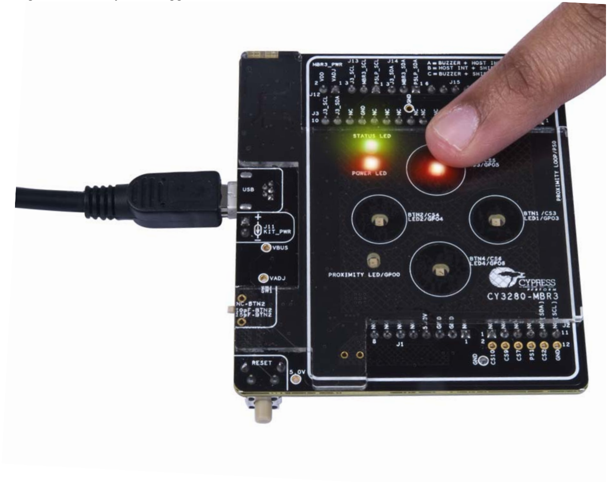
Figure 5-6. Verify LED Toggle Feature
