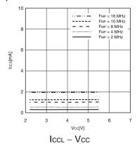
$T_A = +25$  °C,  $F_{MPL} = 16$  kHz (divided by 2) Subclock mode with the external clock operating
