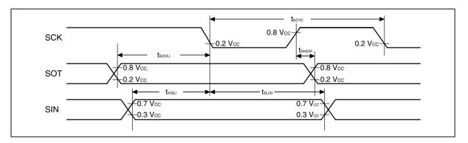
Sampling is executed at the falling edge of the sampling  $clock^{*1}$ , and serial clock delay is enabled\*<sup>2</sup>. (ESCR register : SCES bit = 1, ECCR register : SCDE bit = 1)
