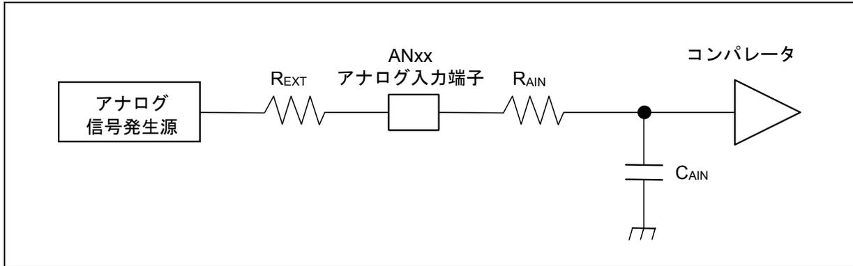
(式 1)  $t_s \geq (R_{AIN} + R_{EXT}) \times C_{AIN} \times 9$
