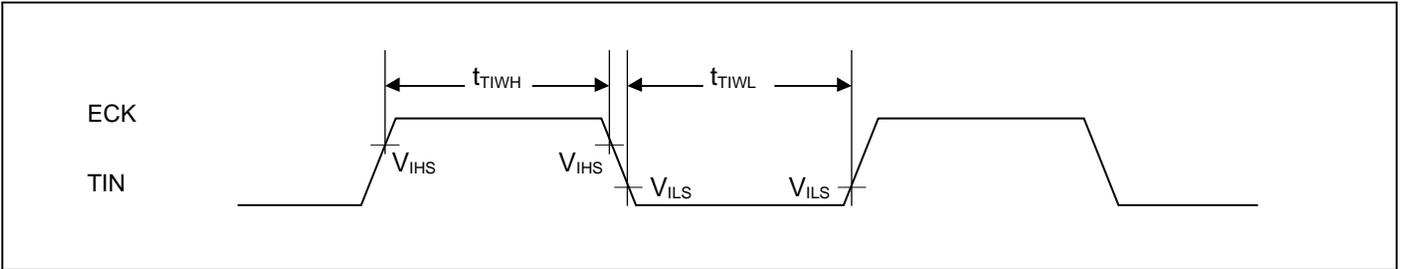
Trigger input timing
