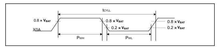
In the case of 48 pin Package, V<sub>BAT</sub> is V<sub>CC</sub>.
