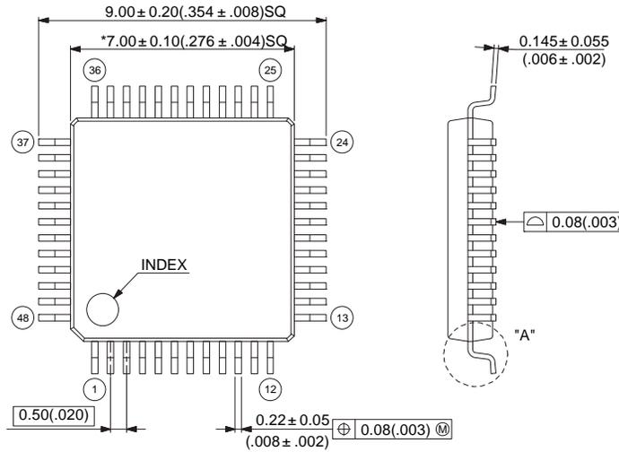
Note 1) \* : These dimensions do not include resin protrusion.
