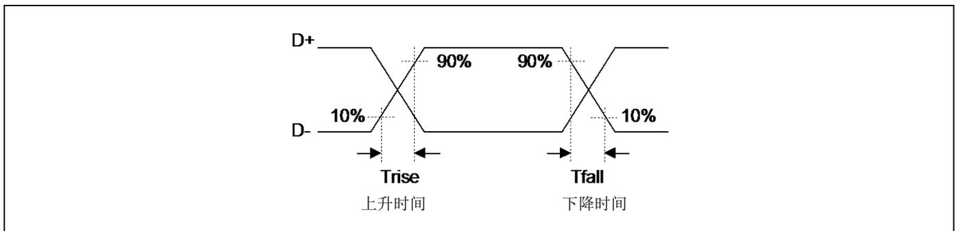
关于外部负载条件, 详情参考"Low-Speed Load (Compliance Load)"
