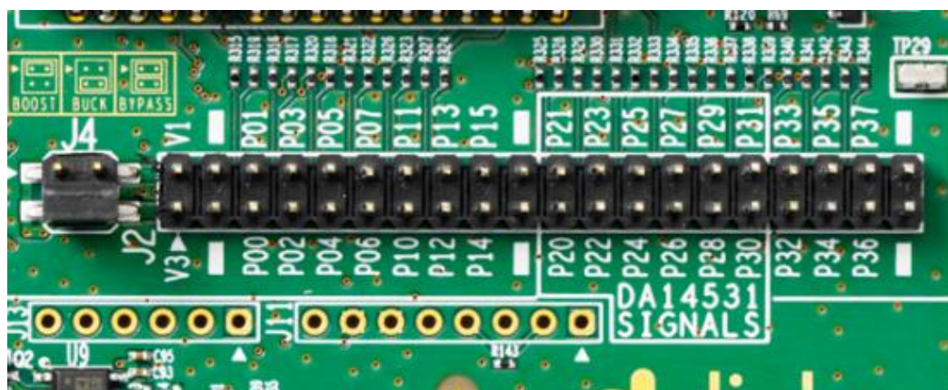
Figure 18: J2, Breakout Header of DA14531 PRO-MB
