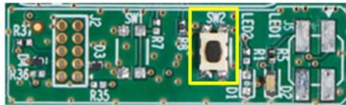
Figure 11: Default general purpose push button (SW2) on DA14531 SMARTBOND TINY™ MODULE DB
