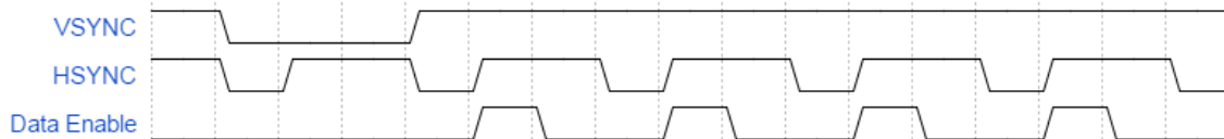
Figure 52: HSYNC/VSYNC Typical Waveform
