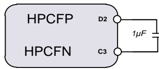
Figure 39: Charge pump flying capacitor
