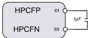
Figure 41. Charge pump flying capacitor
