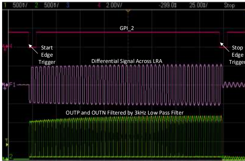
Figure 9: 200 ms Haptic Sequence Oscilloscope Image
