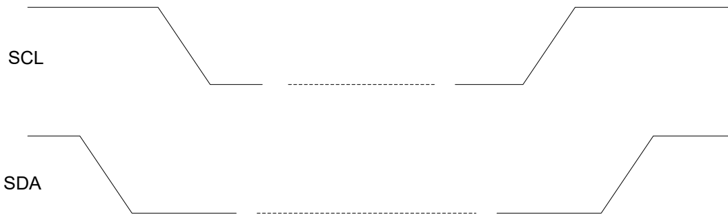
Figure 18: I 2 C START and STOP Condition Timing
