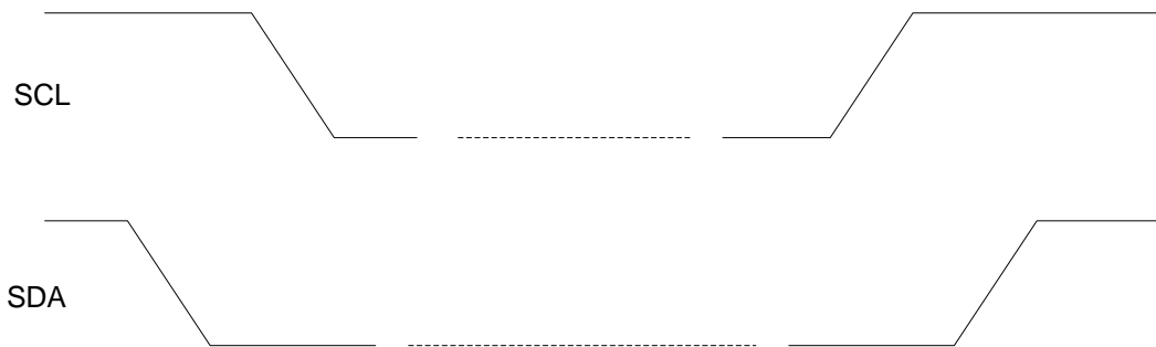
Figure 21: I 2 C START and STOP Condition Timing
