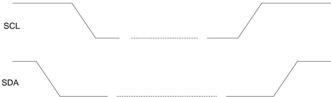
Figure 16: I 2 C START and STOP Condition Timing
