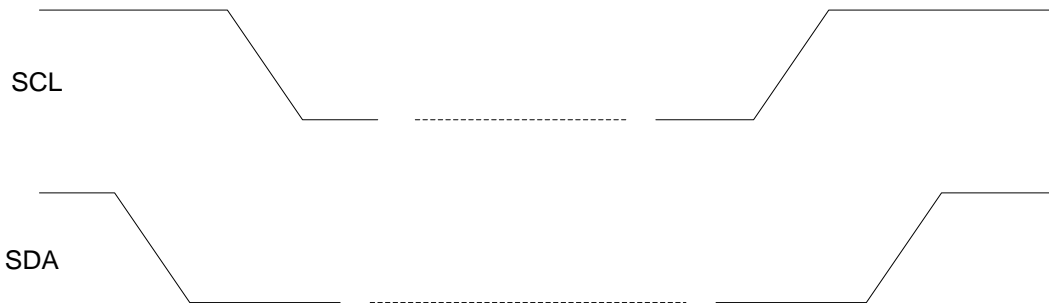
Figure 9: I 2 C START and STOP Condition Timing
