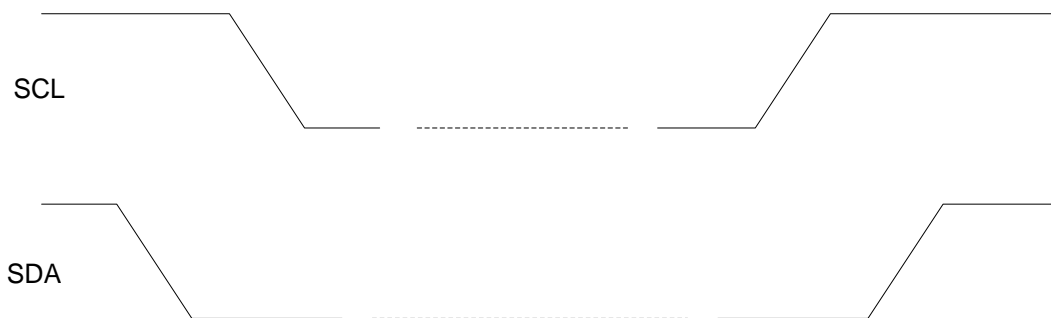
Figure 25: Timing of 2-WIRE START and STOP Condition
