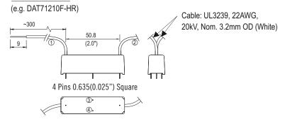
NOTE: PINS WHICH ARE NOT NUMBERED HAVE NO ELECTRICAL CONNECTION.
