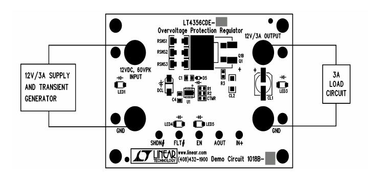
Figure 1: Proper Measurement Equipment Setup
