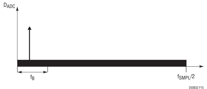
Figure 15. Frequency Spectrum of SAR ADC Core Output
