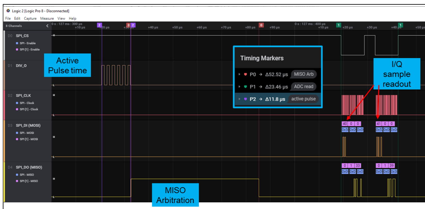
Figure 24 Typical SPI access
