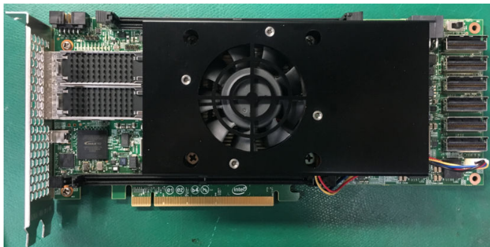
Figure 36. Air-cooled Heatsink Setup
