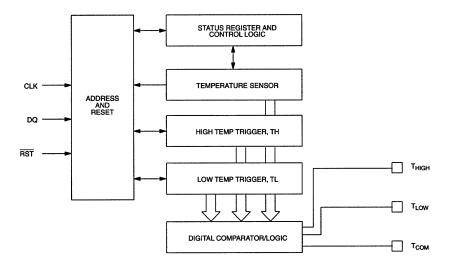
The DS1620 measures temperature using a bandgap-based temperature sensor. The temperature reading is provided in a 9-bit, two's complement reading by issuing a READ TEMPERATURE command. The data is transmitted serially through the 3-wire serial interface, LSB first. The DS1620 can measure temperature over the range of -55°C to +125°C in 0.5°C increments. For Fahrenheit usage, a lookup table or conversion factor must be used.
