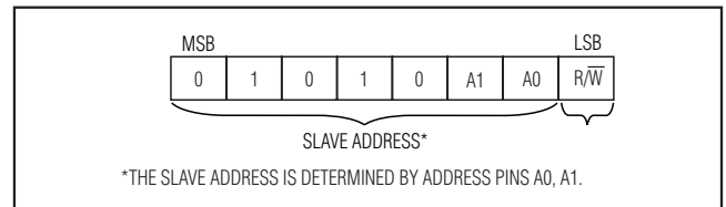
Figure 2. DS3501 Slave Address Byte
