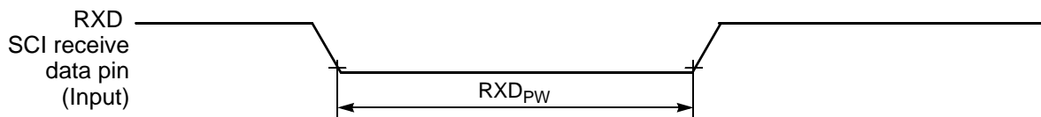
Figure 3-25 RXD Pulse Width
