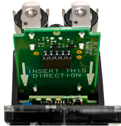
Q45 battery board
