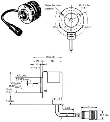
Oil-proof PVC, shielded 12-conductor cable (7/0.18 dia.)
