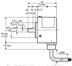
Oil-proof PVC, shielded 12-conductor cable (7/0.18 dia.)
