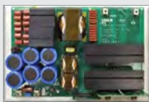
60kW INTERLEAVED BOOST CONVERTER CRD-60DD12N
