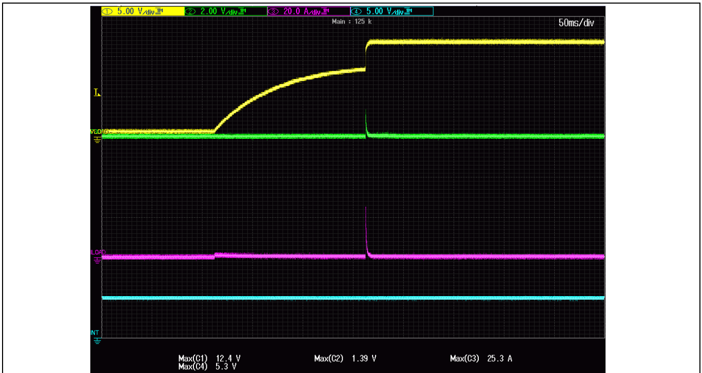
Figure 22 Switching capacitive load with pre-charge [Yellow V_{LOAD} ; Green V_{CS01} ; Purple I_{LOAD} ; Blue V_{INT} ]
