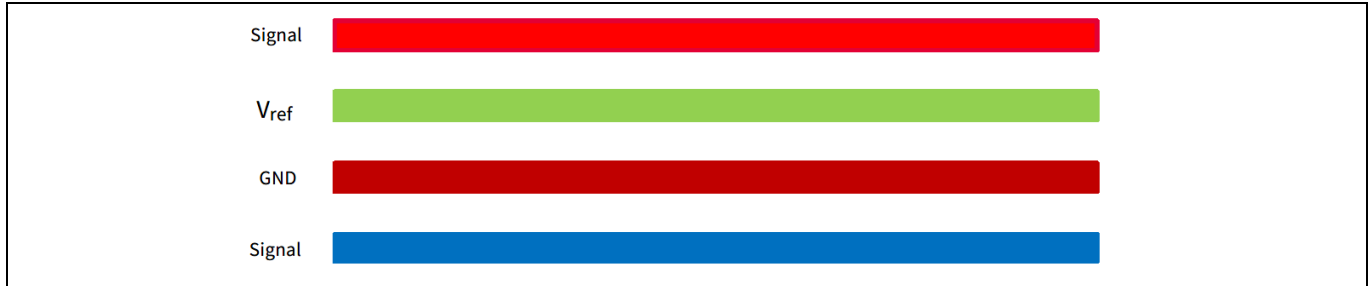
Figure 30 EB 2ED2410 3M PCB layers 4 * 35µm
