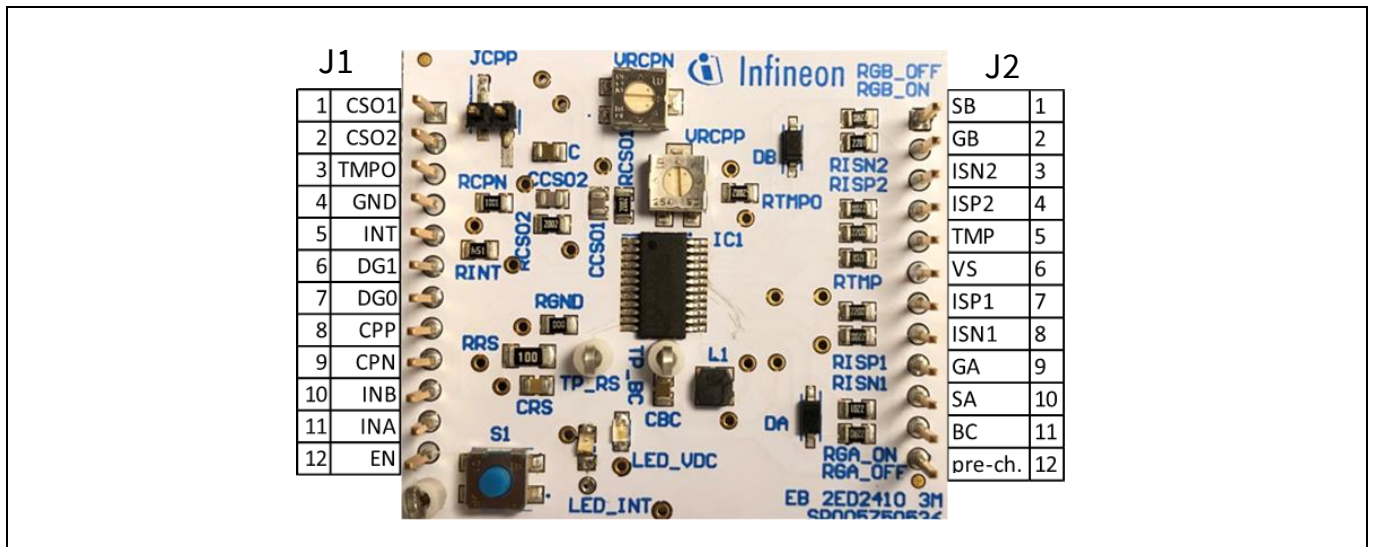
Figure 12 Pin header details with top view
