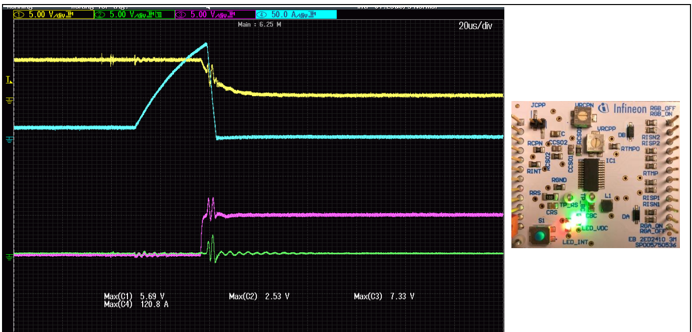
Figure 19 Waveforms from ON to SAFESTATE [Yellow V_{INT} ; Green V_{DG0} ; Purple V_{DG1} ; Blue V_{GS} ]
