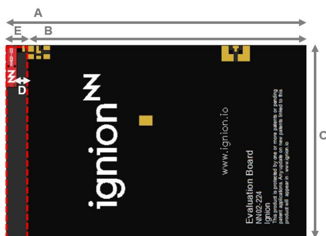
Figure 13 – EB_NN02-224-CR80-2400 in CR80 standard format. Evaluation Board providing operation from 2.4 GHz to 2.5 GHz.
