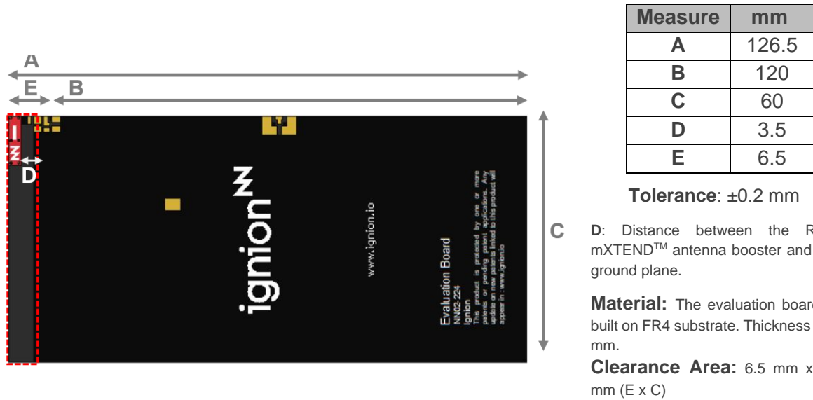
Figure 10 – EB_NN02-224-2400. Evaluation Board providing operation from 2.4 GHz to 2.5 GHz.
