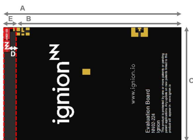
Figure 13 – EB_NN02-224-CR80-2400 in CR80 standard format. Evaluation Board providing operation from 2.4 GHz to 2.5 GHz.
