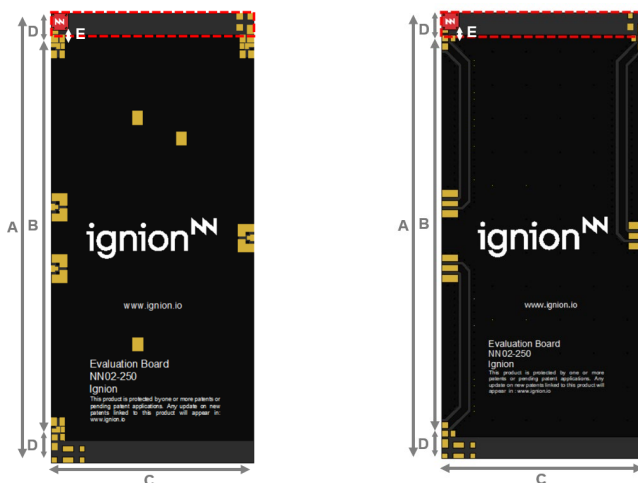
Figure 9 – Evaluation Boards providing operation at LTE1700-LTE2600, 1 port configuration.
