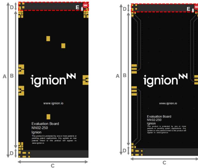
Figure 5 – Evaluation Boards providing operation at GSM850-GSM900, 1 port configuration.
