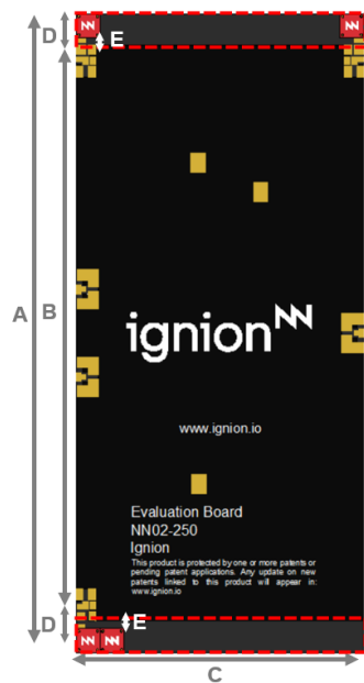
Figure 1 – EB_NN02-250-UFL3R. Evaluation Board with UFL cables. 698 MHz to 798 MHz, 824 MHz to 960 MHz, and 1710 MHz to 2690 MHz.
