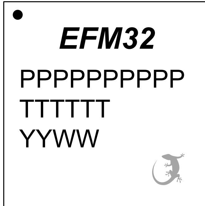
Figure 9.3. BGA112 Package Marking
