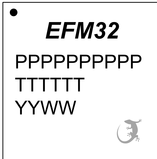
Figure 11.3. TQFP64 Package Marking
