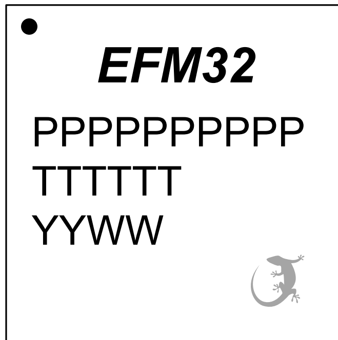
Figure 11.3. TQFP64 Package Marking
